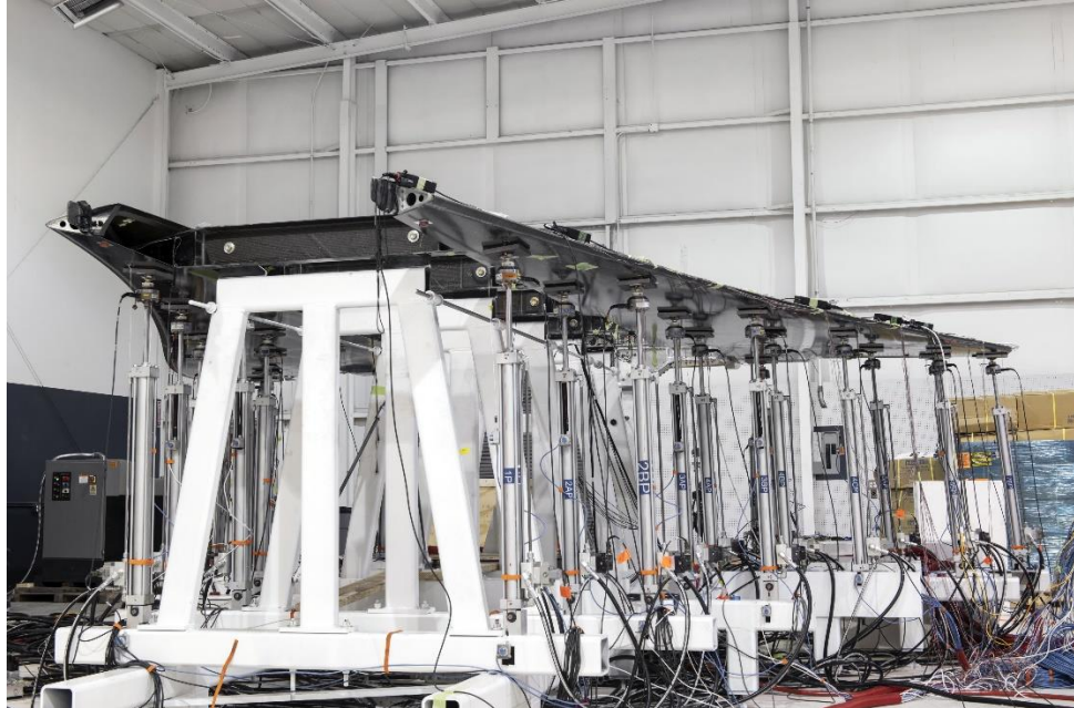
Figure 13. Boom Supersonic's Wing undergoing Load Testing (source: Boom Supersonic)
