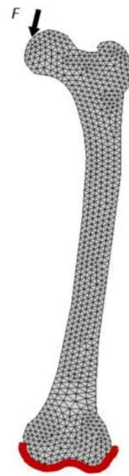
Figure 2. Mesh of Human Femur Bone provided by Colorado School of Mines' FEGN525 Course. Image displays a force being applied in the X and Y directions as well as over 1300 LST elements.
